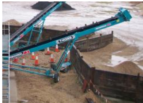
Radial Wheel standard for maximum stockpiling
