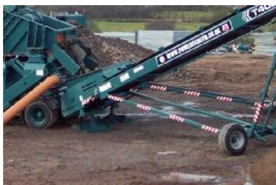
Radial Wheel standard for maximum stockpiling
