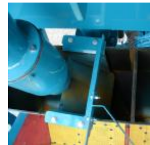
Movable chute to allocate fine material to the coarse product
