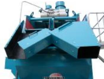
Integrated rubber lined dual chute with blending facility
