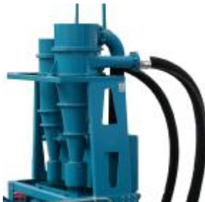
Extended fines cyclone for maximum fines retention
