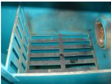
Rubber lined Anti-turbulence inlet
