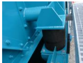
High efficiency rubber screen mount for minimal vibration
