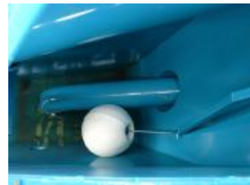
Float system for self regulation of tank water level
